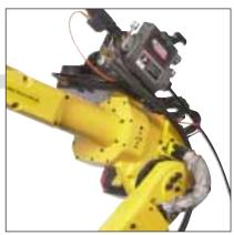
Power Feed 10R mounted on FANUC Robot Arm.
